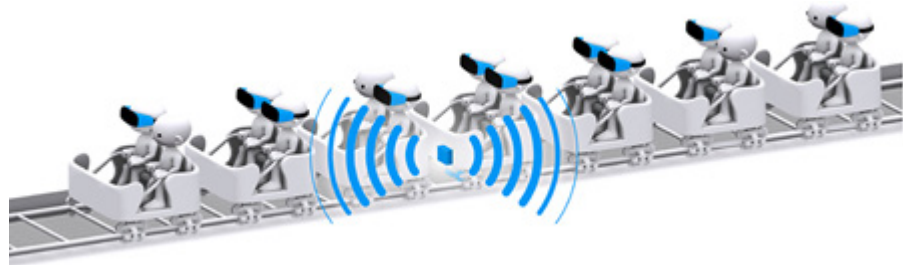
Figure 70. A Single VR Coaster Box Can Sync Any Number of Headsets in Reach.
