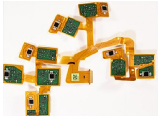
Figure 35. HTC Vive: Infrared Sensors All Over Headset (left), FPC Sporting Infrared Sensors (right)
