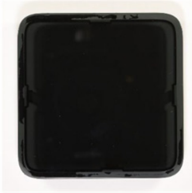
Figure 33. HTC Vive: Infrared LEDs on Base Station, Detects LEDs on Headset
