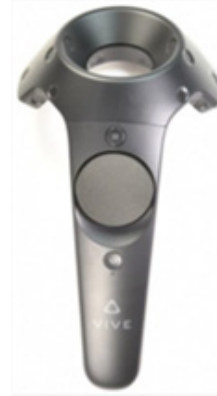
Figure 34. HTC Vive: Controller, Like Headset, has Infrared Sensors
