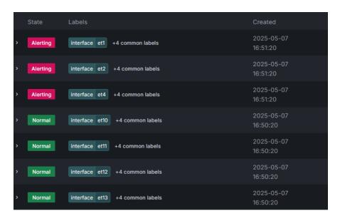
Example of the alerting section of Grafana, showing the 3 interfaces on which we sent CST packets (et1, et2 and et4) breaching the defined threshold.
